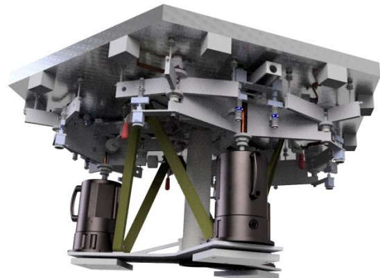
Fig. 5 Conceptual design of the M1 Segment Subunit (Image: ESO)
